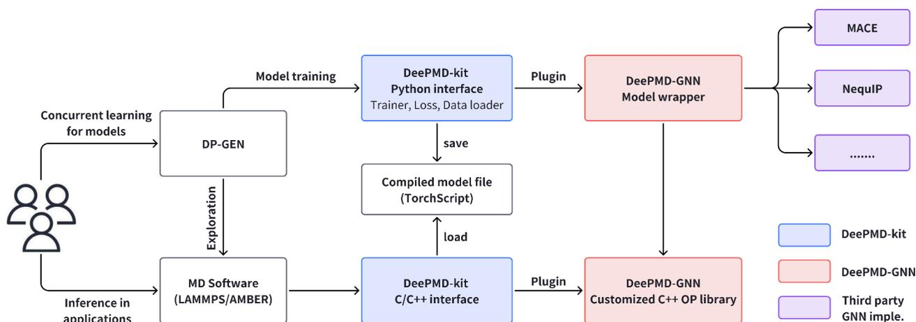
**Figure 2.** Software architecture of the DeePMD-GNN package. The boxes represent software components, and the arrows represent dependency between the software and the flow of data.  $A \rightarrow B$  means that software component A depends on B; A calls B with input data, and B returns the output back to A.
